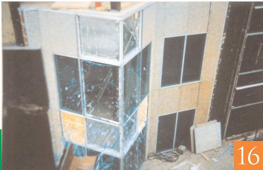
Fig. 19 – Glass Failure during Curtain Wall Testing
